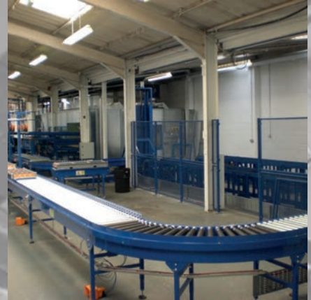
PPL Tufthane Logistics System incorporating powered rollers, overhead chains and heavy duty towing conveyor.
